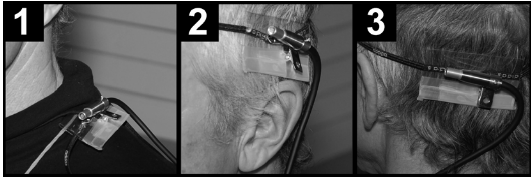
Figure 2: The different tested microphone positions, 1 = on the shoulder, 2 = above the ear, 3 = on the back of the head
